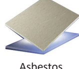
Asbestos Mill Board
